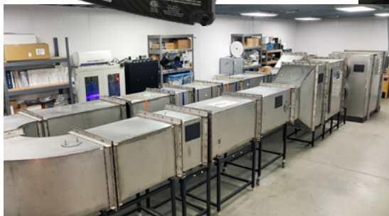
In-house ASHRAE 145.2 Test Chamber
